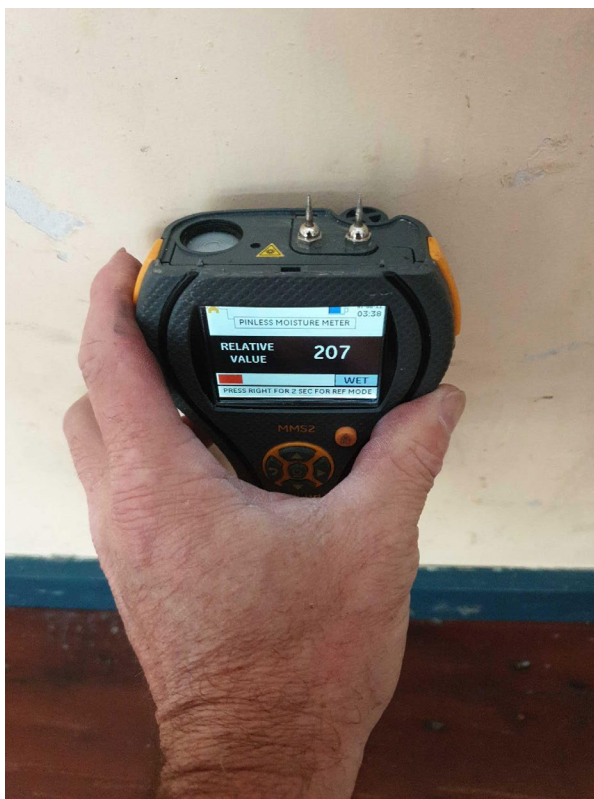
Figure 15 - Much of the lower wall presented high moisture readings
