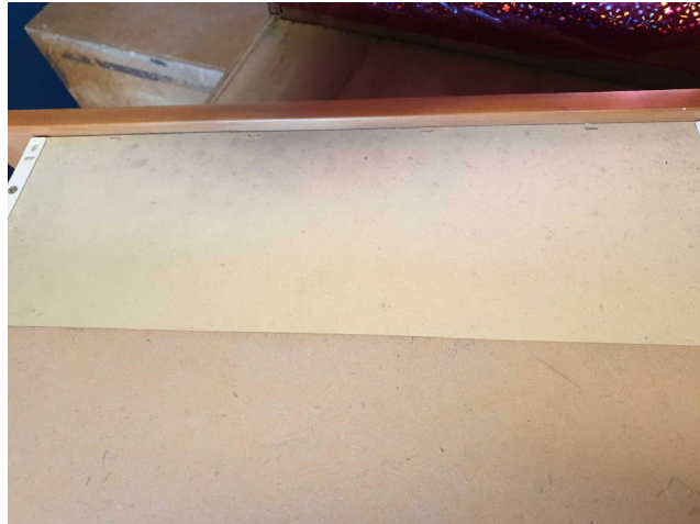
Figure 44 - Some unfinished timbers such as the bottoms of draws on desks in the storage area are deemed to be unsalvageable
