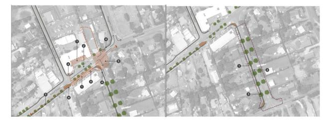
**Section 6** – Section 6a will primarily be developed through Mangawhai Community Park with connections across Molesworth Drive connecting to the east side. This will include a new shared path on the eastern side, connecting with existing footpaths, from ITM through to the bridge.
